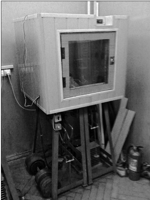
Fig. 1. Cooling chamber and uniaxial compression systems.
