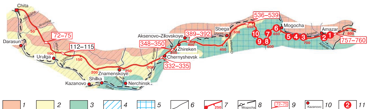
Fig. 1. Geocryological and geomorphic setting along the Amur federal motor road in Transbaikalia [Kontrat'ev et al., 2010].
