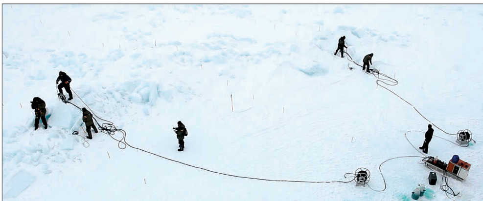
Fig. 2. Overview of the UVBL-2 thermal (hot-water) drilling system for ice drilling.
