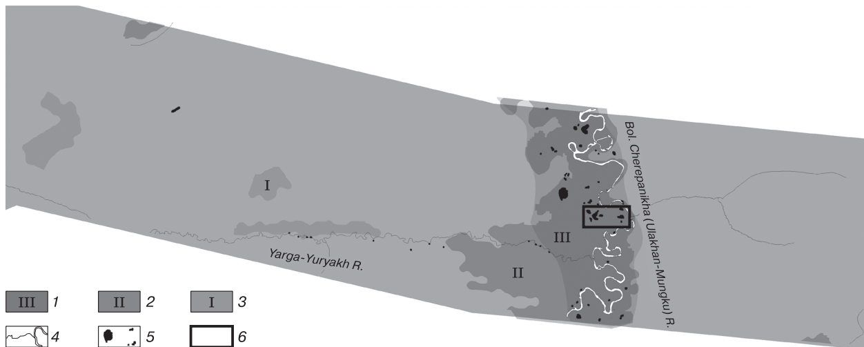
Fig. 2. Fragment of the zoning map of buffer area of the trunk oil pipeline at the intersection with the Bolshaya Cherepanikha River according to conditions of thermokarst development:
