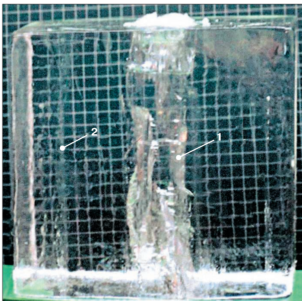
Fig. 5. Deformation upon quasi-static indentation:
